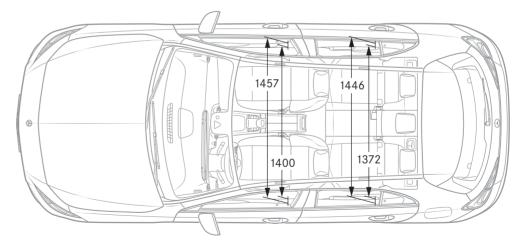
All figures in millimetres. The dimensions shown are average values. They are valid for vehicles in basic specification and in unladen condition.
